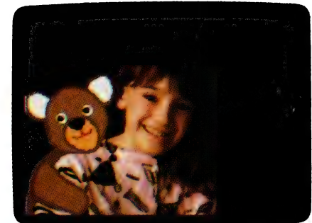
Using the Apple Video Overlay card is straightforward – first, create the graphic, then select VideoMix from the menu, cue the video source to the sequence to be overlaid, play it, and begin recording with a second VCR.
